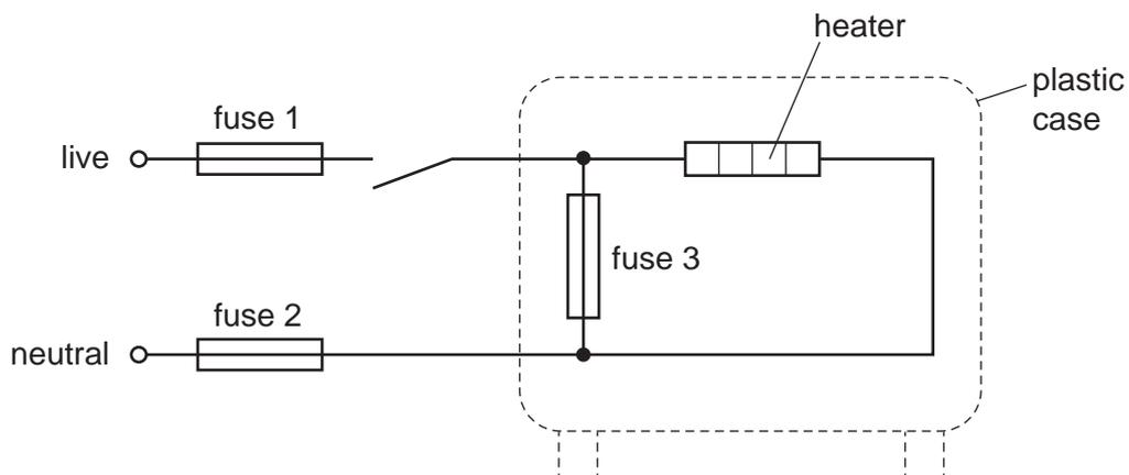
Which of the fuses are correctly placed?
